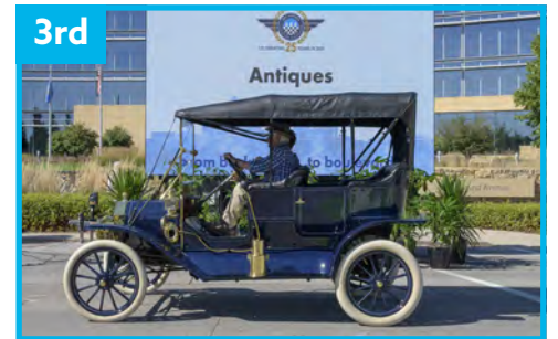
3rd 1911 Ford Model T owned by John and Karen Goedeken of Palo, IA. This early 1911 Ford Model T, the 64,488th built, predates the assembly line. This "touring" model originally sold for $780.00. As a "brass car," it boasts brass trim before wartime needs shifted to steel, creating "black T's." Lighter and more powerful with higher compression, these early T's were simple, sturdy, and competitive.
