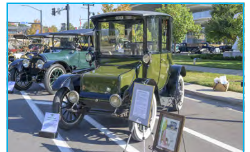
1916 Rauch & Lang owned by Bob Gerdes of Burlington, IA. Makers of electrically powered automobiles from 1905, Rauch & Lang of Cleveland, Ohio had previously been active in the carriage trade. This model has tiller steering from the rear seat, and can seat three, with the front seat turned towards the rear. Cruising speed is 20 mph with a range of 50 miles, from 14 batteries.
