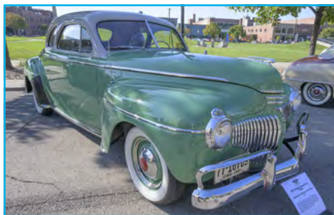
1941 DeSoto Custom Club Coupe owned by Dave Holzinger of Des Moines, IA. In 1941, DeSoto introduced the vertical bar grille which became its styling theme through 1955. Advertised as having "Rocket Bodies", the new styling, combined with Chrysler Corporation's engineering, made 1941 the highest sales year to date. This was the first year DeSoto offered Chrysler's Fluid Drive semi-automatic transmission.
