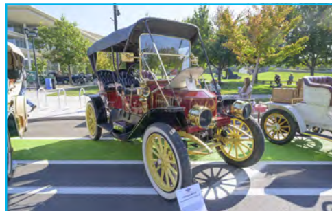
1909 Stanley Model R owned by Michael Curry of Cumming, IA. The 1909 Stanley Model R, with its red wooden body and gleaming brass, showcases steam power's golden era. Restored in 1996 by specialist Jim Keith, it features a 20-hp twin-piston engine with only 13 moving parts. It's toured extensively—including 5,300 miles from Alaska to Maine—Powered by a kerosene pilot, Jet-a Main and water.
