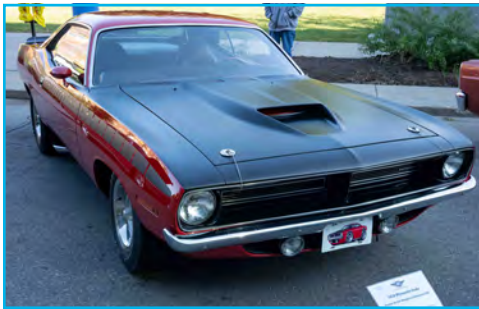
1970 Plymouth Cuda owned by Jim Wesanto of Nashauk, MN. This AAR Cuda is one of 2724 built to compete in the Trans-Am racing series. The unique features include wider tires in the rear, 4 speed manual transmission coupled to a Hurst close ratio shifter, special side exit exhaust and a fiberglass hood held down by only hood pins.
