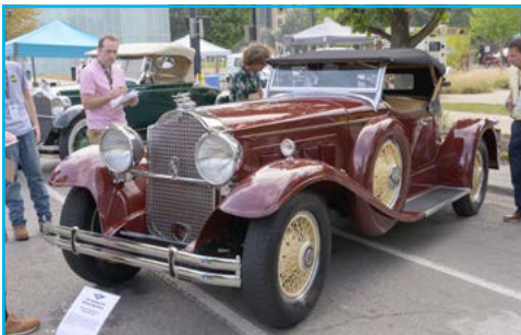
1930 Packard 734 Boattail Speedster owned by Winston Peterson of Golden Valley, MN The Packard Speedster Eight was one of the first cars to use the muscle car recipe: a lightweight body mounted on the company's shortest chassis and fitted with a modified version of its biggest engine. The limited edition (39 built) Speedster was thought to have been developed to race at LeMans, but that never occurred.
